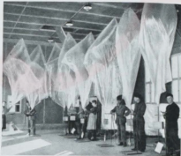
Production line for large plastic balloons. Paperboard containers attached to balloons carry the computed weight of paper. Below the container, a paper envelope holds dry ice ballast which permits timing of the release of the leaflets.
