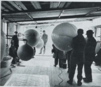
Production line for rubber balloons. Exact amount of hydrogen is measured by the balancing on an arm on the filling device, an invention of Czech member of Free Europe Press. Workers seal filled balloons with leaflets inside.
